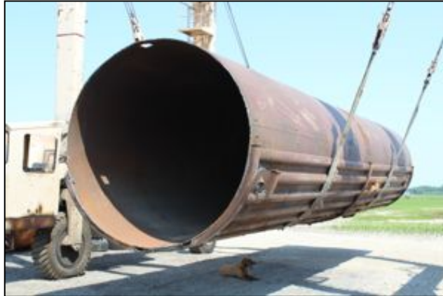
Figure 40: Tank car with tank end and wheel trucks removed
